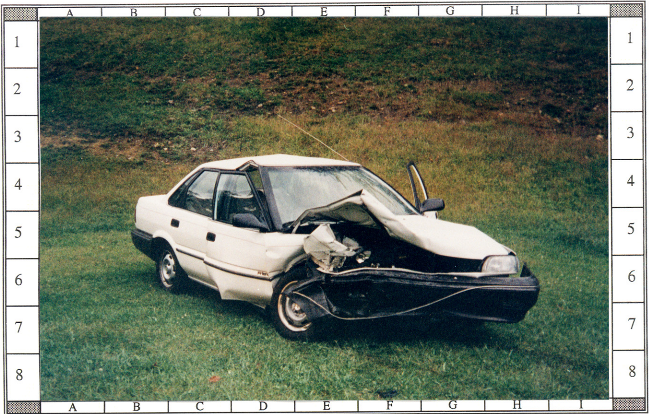
# 07: On scene westward view of Vehicle #2 at final rest (heading northeast) showing severe frontal damage, roof buckling, and induced damage to right front door
